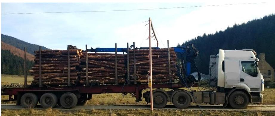
Re-construction Pic 1. Crane positioned within central trough in the timber load
