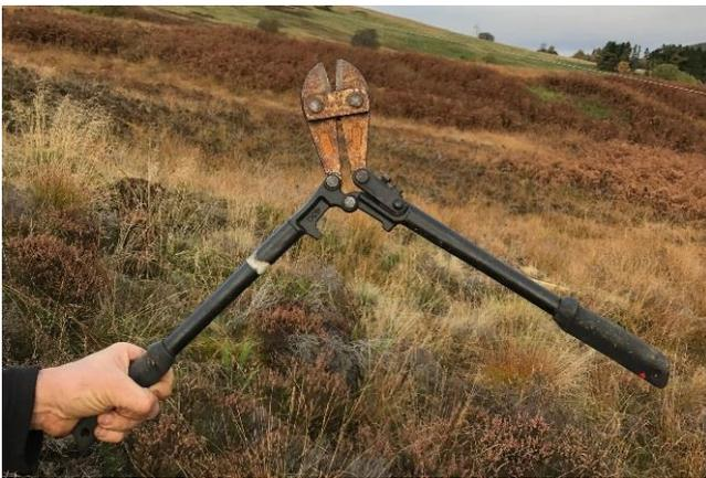
The operator was bending over cutting one of the bottom wires with a set of bolt cutters when one of the sections of wire sprang up and caught him in the right eye.
