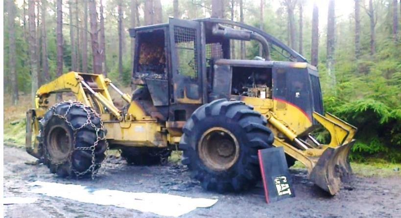
Starter motor, alternators, air conditioning units and the associated wiring, - rank high in the initial cause of machine fires.
