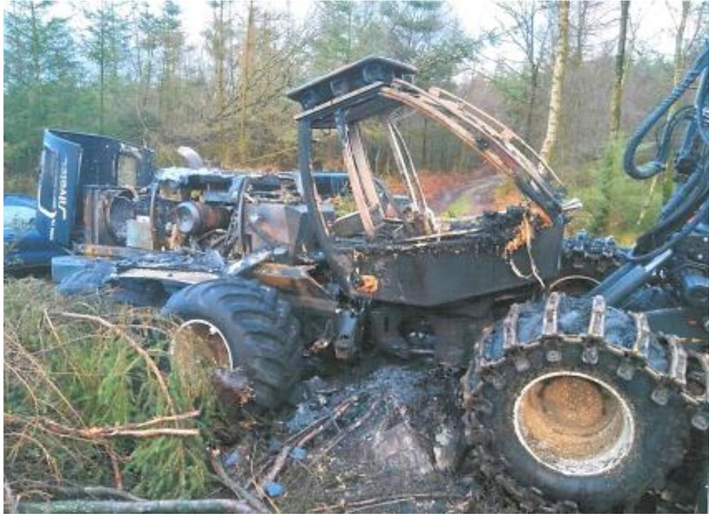
the smoke ignited at that point. The machine's automatic fire suppression system activated, and the operator used his hand-held applicator to try to extinguish the flames. The fire was quickly out of control. The operator retreated a safe distance and called the fire brigade.
