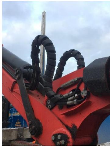
If one of the pipes burst in the jib extension, consider replacing the parallel pipe, it is likely to have been damaged or degraded to the same extent as the failed one.
