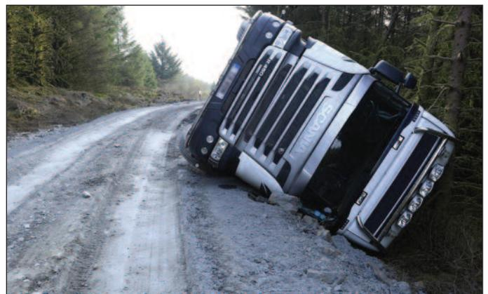
The vehicle was recovered using two heavy recovery vehicles with winch and pulley systems working to a Dynamic Risk Assessment. The vehicle was not restarted and was towed away on a suspended lift.
