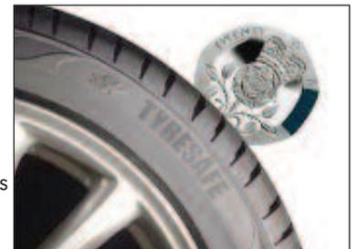
To test, take a 20p and place it in-between the main grooves of the tyre. If you can see the outer band of the coin, the tyre may have insufficient tread depth. At this point, it is advised that you have your tyres checked over by a qualified mechanic.
